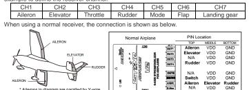
When using a DSM/S.BUS receiver, OUT1, OUT2 and OUT4 channels are respectively connected to aileron, elevator and rudder, and OUT3 is connected to the ESC. OUT5, OUT6 are used to respectively output the CH6 and CH7 signal of receiver and connect with flap and landing gear. The connection is shown as below:
